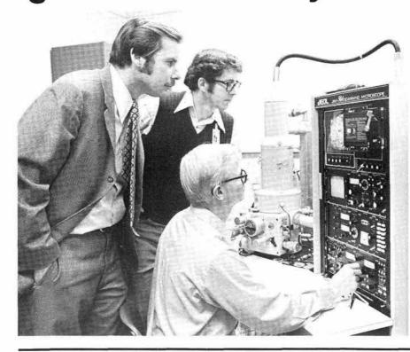
SCANNING ELECTRON MICROSCOPE reveals extent of hydrogen embrittlement of a test specimen. Jim Swisher and Steve Robinson (both 8313) study test results on video screen. Operator is Clarence Karfs (8312).
